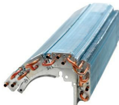
Evaporator Coil (indoor coil) from a Split System. The coil employs 5-mm diameter MicroGroove copper tubes, which resulted in a 30 percent reduction in tube weight for the same performance (2500W cooling capacity) as previous models.
